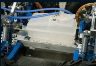
This oversize fuel tank will ensure that my rig runs for a long time. I made the custom mount out of diamond plate aluminum and a couple of standoffs.
