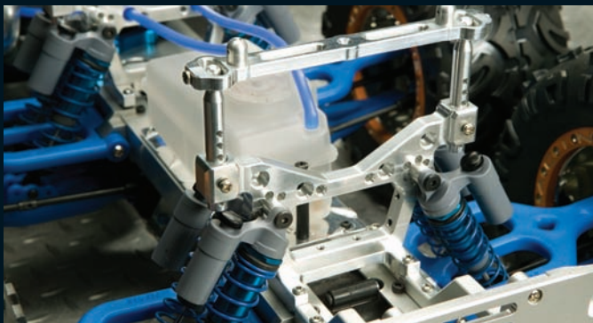
These good-looking shock towers are also tough. New Era gives you more shock-mounting holes so that you can fine-tune the suspension.
