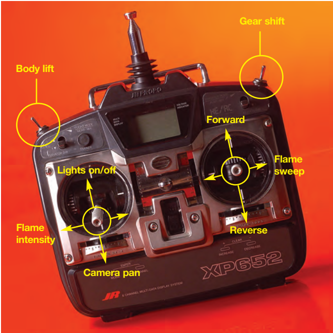
You can use any radio to control this truck's actions. Scott uses a JR 6-channel radio for the job at hand. It controls 10 functions!
