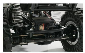
and unlocking the differentials easy. Simply remove a threaded pin, and the locked diff becomes an open diff. The axles and the rest of the drivetrain spin on included ball bearings.
