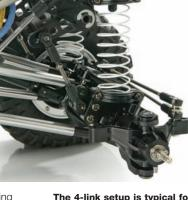
The 4-link setup is typical for a rock crawler, but the remotely mounted coil springs and cantilevered shocks are quite distinctive.
